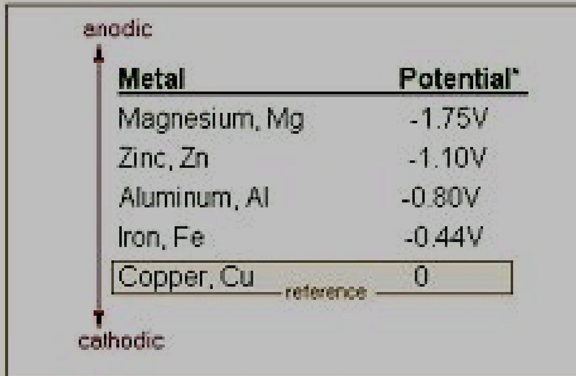
The diagram shows a vertical list of metals with their corresponding potentials. A vertical arrow on the left points upwards, labeled 'anodic' at the top and 'cathodic' at the bottom. The metals are listed from top to bottom: Magnesium, Mg (-1.75V); Zinc, Zn (-1.10V); Aluminum, Al (-0.80V); Iron, Fe (-0.44V); and Copper, Cu (0). The Copper, Cu entry is enclosed in a rectangular box and labeled 'reference' below it.
